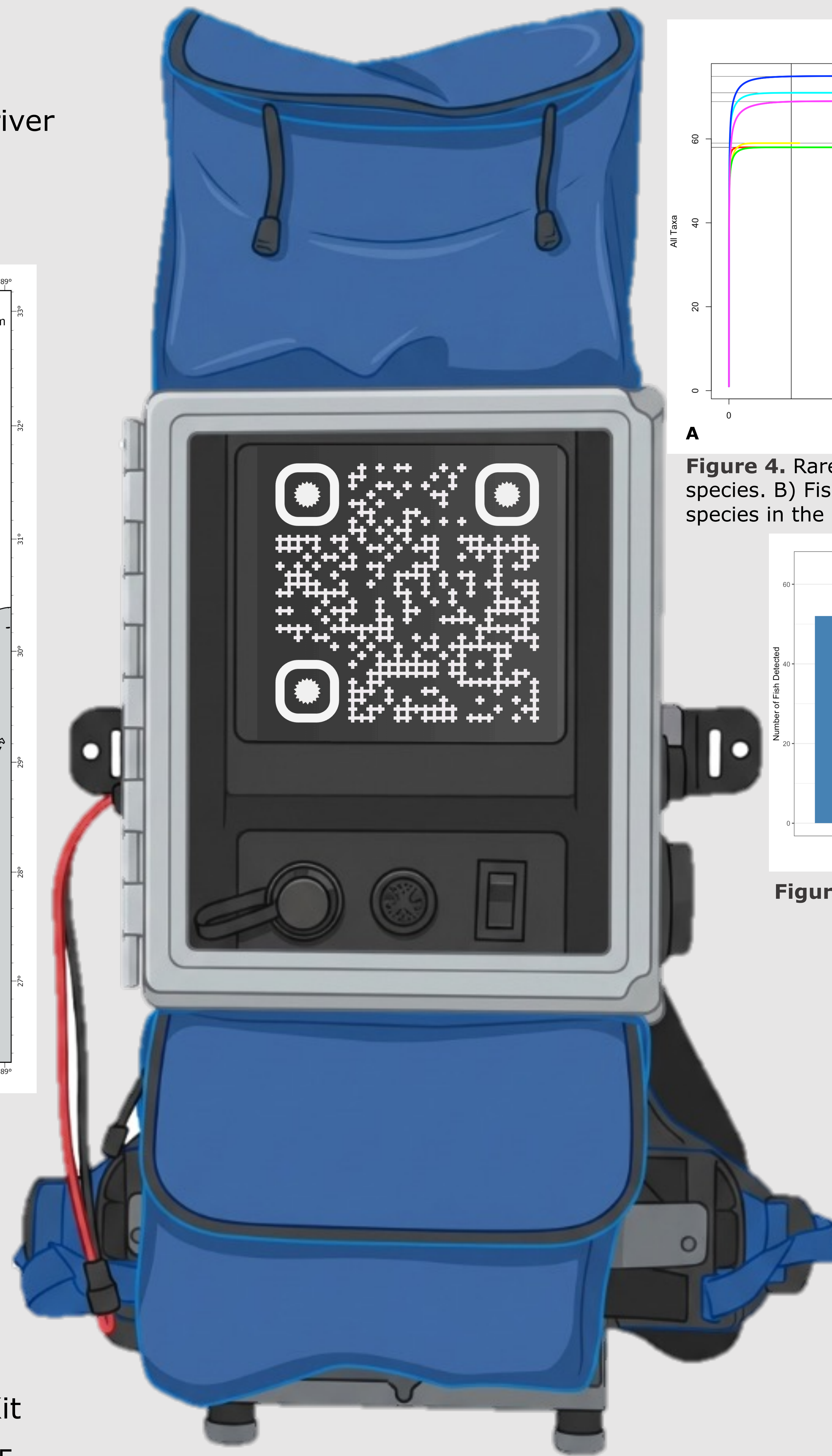
Figure 3. Smith-Root eDNA Backpack Sampler. Use the QR code to see the what species were detected!
